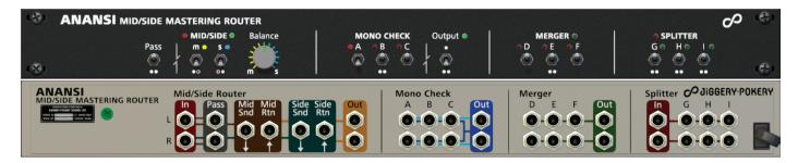
Anansi is an audio router that has been designed for use in your Master Inserts chain, in particular for controlling a mid/side processing chain.
